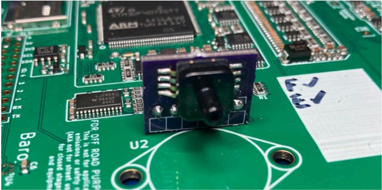
Using the MAP line combined with an intake air temperature (IAT) sensor, the BMM ECU can run the car using what is known as speed-density air metering. This means that you can unplug the mass air flow (MAF) sensor or the air flow meter (AFM) for the NA 1.6L vehicles. Removing these sensors and replacing them with a pod filter directly to the intake can even result in a fractional power increase from the reduction in intake restriction.
