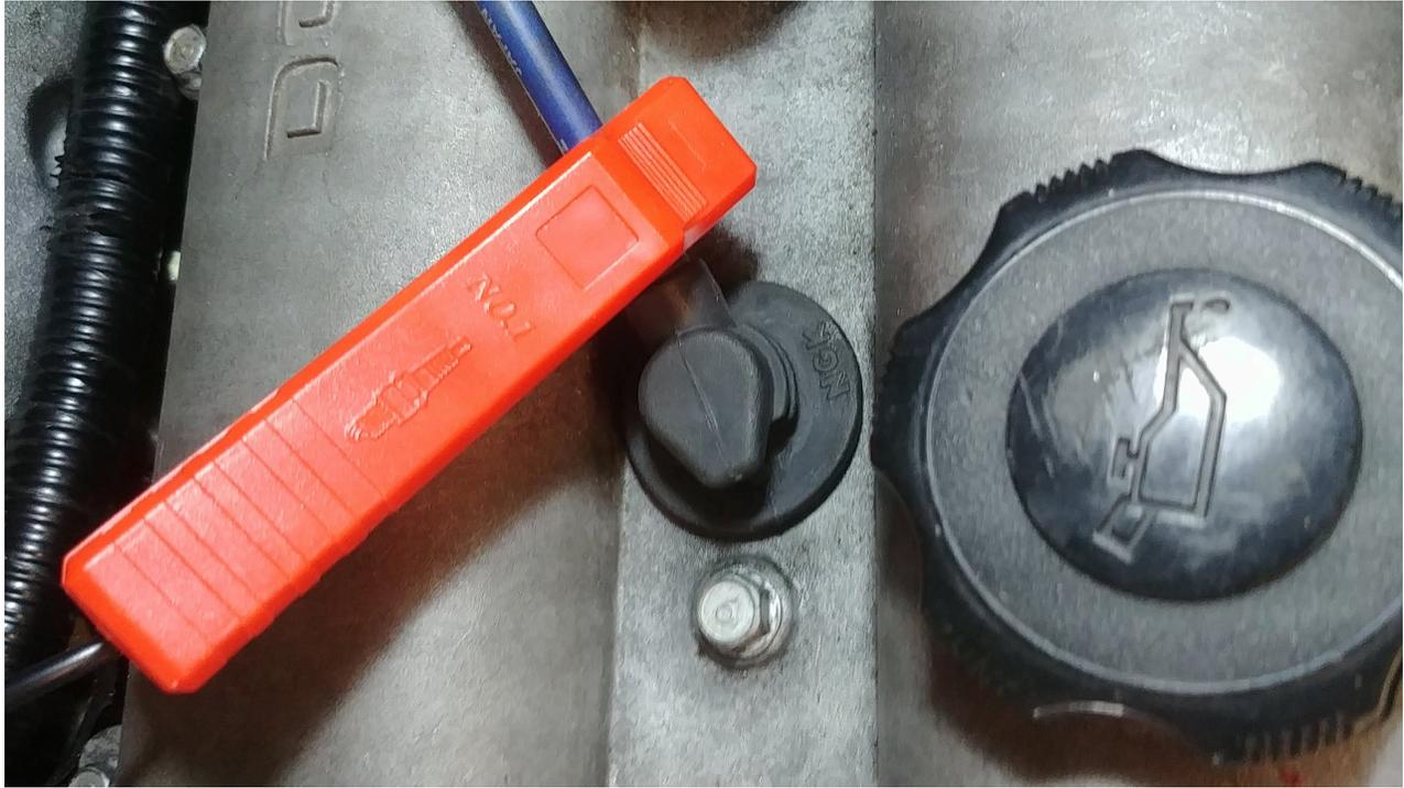
In TS, under *Ignition > Ignition Settings*, set the timing mode to *fixed* and *10* degrees then burn the configuration.
