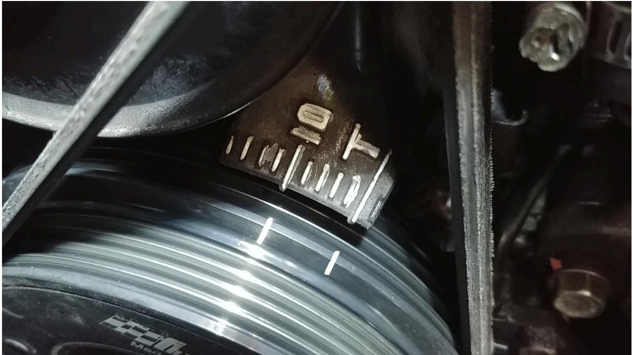
If your timing marks do not line up like in the image above, you will need to change the base timing. Count how many marks the timing is off by and turn the car engine off. In TS, go to *Base Engine > Trigger* and increase/decrease the *Trigger Advance Angle* by the amount of marks the timing was off by then burn the configuration. Repeat this process until the timing marks line up then change the timing mode back from *fixed* to *dynamic*.
