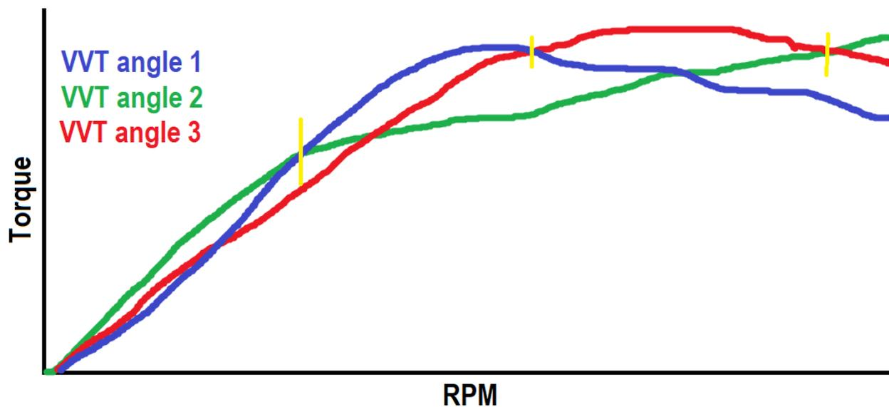
If you have some way of maintaining a constant throttle position below 100% such as a chock under the pedal (**on the dyno only!!!**) or limiting the maximum throttle body travel, ramp runs can be used to efficiently populate the whole VVT table for conditions where the engine isn't fully
