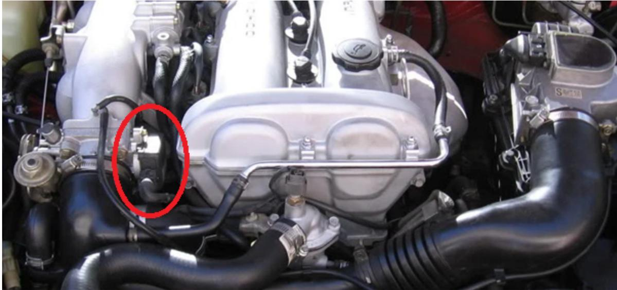
The BMM ECUs for this vehicle include a KIA TPS and adapter. The KIA TPS will plug straight to the OEM TPS plug without any additional wiring. If using another variable TPS that requires re-wiring, the NA6 TPS connector pinout is as follows:
