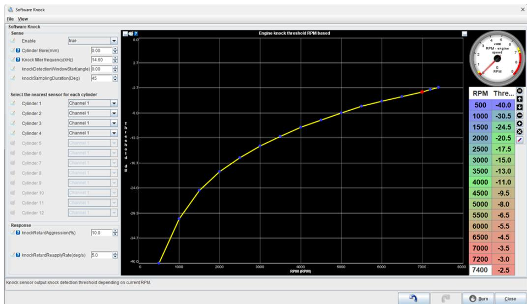
6. Set up the Response of the Knock controller's parameter "Knock retard aggression" A generalized rule of thumb would be
