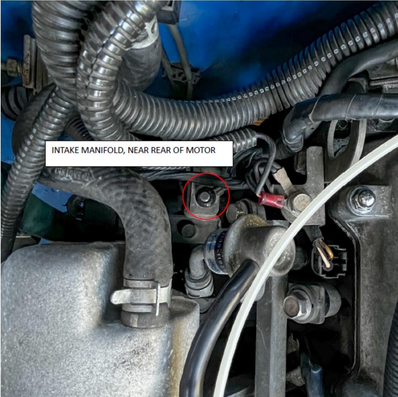
INTAKE MANIFOLD, NEAR REAR OF MOTOR
