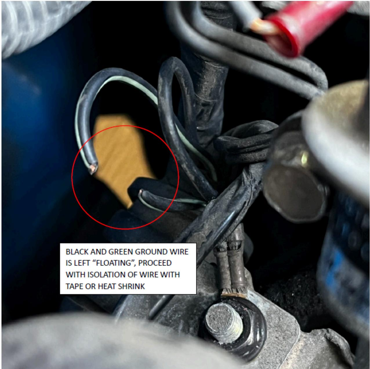
Note: If your car's ground is different due to modifications, follow the harness from the passenger side firewall to the cam angle sensor, and the pair of grounds may have been relocated to another location. See the NA6 wiring diagram at the end of this guide for further information.
