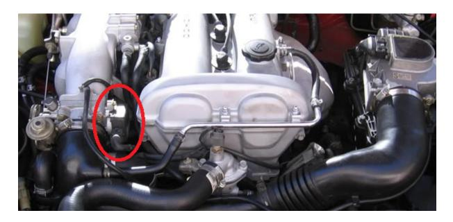
The BMM ECUs for this vehicle include a KIA TPS and adapter. The KIA TPS will plug straight to the OEM TPS plug without any additional wiring. If using another variable TPS that requires re-wiring, the NA6 TPS connector pinout is as follows:
