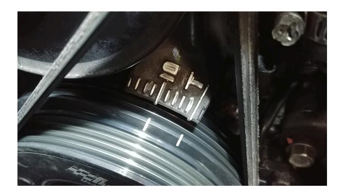
If your timing marks do not line up like in the image above, you will need to change the base timing. Count how many marks the timing is off by and turn the car engine off. In TS, go to *Base Engine > Trigger* and increase/decrease the *Trigger Advance Angle* by the amount of marks the timing was off by then burn the configuration. Repeat this process until the timing marks line up then change the timing mode back from *fixed* to *dynamic*.
