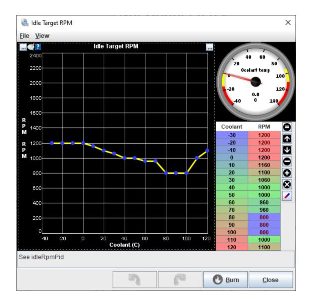
Defines the target idle RPM used by the main Closed Loop Idle air strategy as well as *Closed Loop Idle Ignition Timing*. Log variable is *Idle: Target RPM*.
