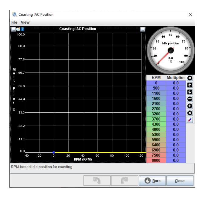
Only enabled when *Use coasting Idle Table* is set to **true**. 2D Table. When the engine is in the *coasting* phase, the IAC base position is set to the value defined by this table. This table is not used if the engine is not in the *coasting* phase and the *open loop base position* will be used instead.
