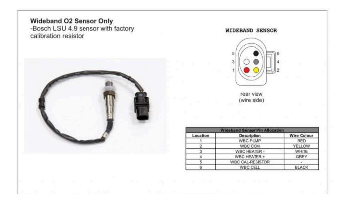
**Note:** The calibration resistor is internal to the sensor. On the sensor connector, there are only 5 wires but 6 pins, as pins 1 and 5 have a laser-trimmed resistor between them.
