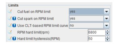
Hard cuts apply when an engine reaches the *RPM hard limit*. In most cases, it is recommended to use fuel cut instead of spark cut.
