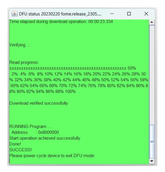
If the update completes successfully, congratulations; proceed to the Setting up TunerStudio section. If the update does not complete successfully, the firmware may need to be loaded by first forcing the board into bootloader or Device Firmware Update (DFU) mode, documented in the next section.
