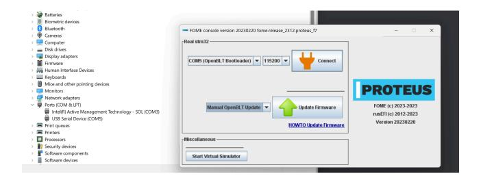
If prompted with "Update completed successfully!", proceed by power cycling the ECU. From this release onwards the ECU can be updated using OpenBLT and should not require any manual driver installs.
