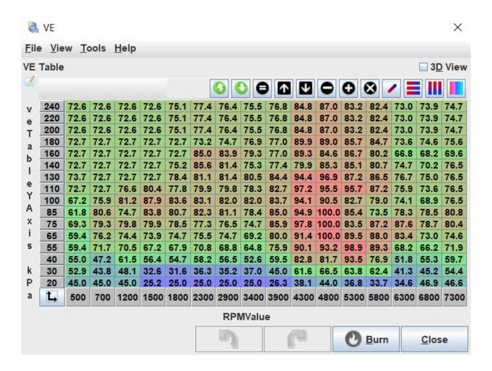
The general way to tune the VE table is to go through all the cells which the engine will operate within and to adjust the VE percentage until the lambda gauge matches the value in the *Target Lambda Table* shown below and in TS found under *Fuel* > *Target Lambda*. For example, if the lambda gauge shows 1.1 and the target lambda for that engine state is 1.0, the corresponding VE cell needs to be increased by 10%. The target lambda table supplied with the Miata base map should be sufficient to
