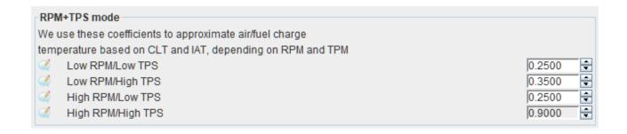
For example, a coefficient of 0.2500 means that 25% of the estimated air temperature is from the IAT, and 75% from the CLT. If the IAT was 40C and the CLT was 80C, the calculation for estimated air temperature would be (40C \* 0.25) + (80C \* 0.75) = 70C.
