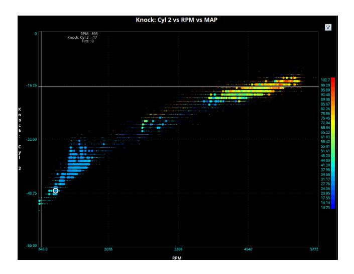
The normal noise scatter plot also has a significantly better (higher) signal-noise ratio than the knocking plot above. Independent of the knock events, noise levels occur in a smaller range and the vertical size of the "band" across all RPMs is much smaller. The smaller vertical distance can be interpreted as noise levels being more consistent.
