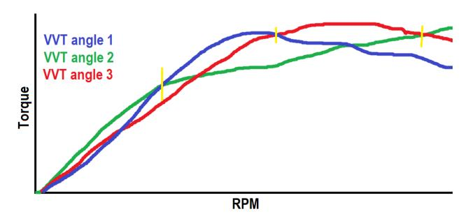
If you have some way of maintaining a constant throttle position below 100% such as a chock under the pedal (**on the dyno only!!!**) or limiting the maximum throttle body travel, ramp runs can be used to efficiently populate the whole VVT table for conditions where the engine isn't fully
