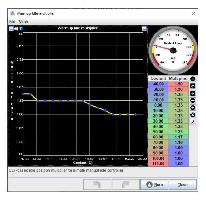
The *open loop base position* value is multiplied by the value in this table. For example, if the *open loop base position* value was 30% and the multiplier was 1.50 at 0 degC, the commanded base position at 0 degC would be 45%. A multiplier of 1 would simply output the open loop base position value.
