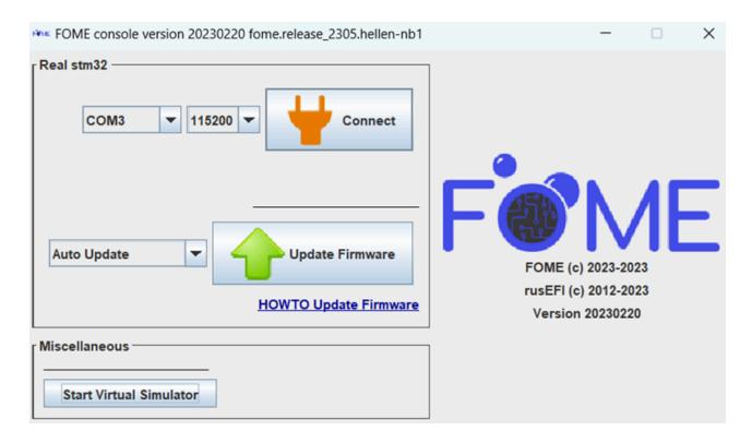
Next, choose the *Update Firmware* button and leave the board connected until the console notifies that the update was successful with a green display. Only once the console has presented this success message, disconnected and re-connect the ECU to the computer to reboot it with the new firmware.
