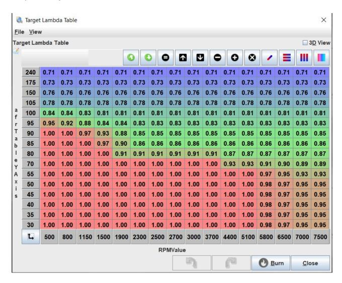
There are three ways of tuning the VE table. The first way is to drive the car around smoothly as a mate in the passenger seat goes through and changes the VE values until the lambda gauge matches the target lambda. The second and easier way is to use the TS autotuner which is only available in the full version of TS but absolutely worth it. To tune this way, you first need to disable some parameters. Under *Fuel*, open *Closed*
