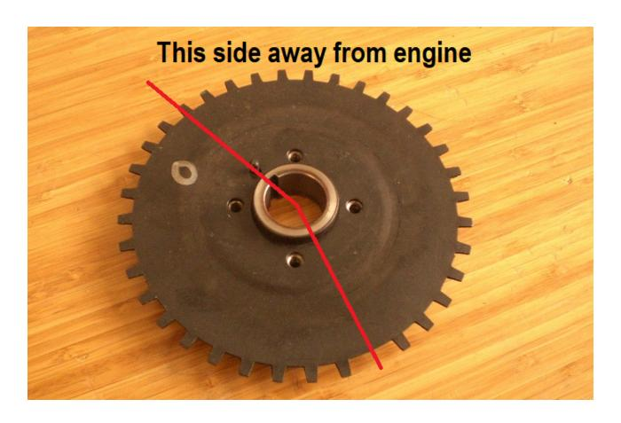
If installing an ATI damper and trigger wheel or a Fluiddampr, consult the manual as the installation has several additional steps which include
