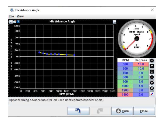
Only enabled when *Use idle ignition table* is set to **true**. 2D table (curve). The values in this table are used in place of the regular ignition curve when idle is active, or during the cranking taper if *Use idle tables for cranking taper* is set to **true**. Unlike *Closed-loop Idle Timing*, this table does not react to *Idle target RPM* and is open loop only.
